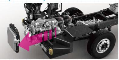
Overhauls and other engine maintenance that were difficult due to the front-engine layout are now easier to perform because the engine can now be easily lifted out of the front area by removing the front cross-member. This helps make maintenance considerably easier to perform.
